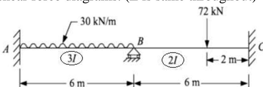
The diagram shows a continuous beam ABC. Support A is fixed, support B is a roller, and support C is fixed. The beam is divided into two spans of 6 m each. The left span AB has a uniformly distributed load of 30 kN/m and a moment of inertia of 3I. The right span BC has a point load of 72 kN at 2 m from C and a moment of inertia of 2I.
